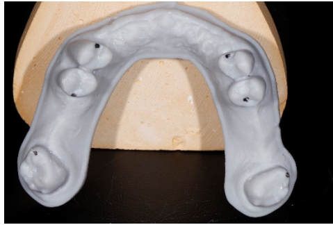
Figure 17: A 3D printed model, printed from intraoral scan data using grey Straumann® P Pro cast resin.
