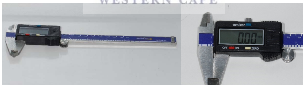
Figure 13c: Blue-Point ® , MCAL6A digital vernier calipers calibrated to two decimal points (mm).
