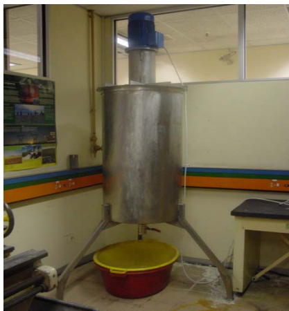
Figure 5.8: Large scale mixer with 250 l tank capacity and turbulator/aeration unit.
