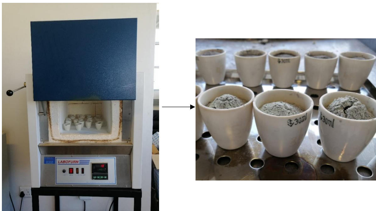
Figure 3.6: Image of alkali fusion samples which were roasted at a 1:1 ratio, 400 °C for 120 min.
