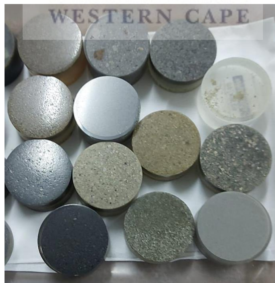
Figure 3.3: Image of CFA samples prepared for TIMA analysis.
