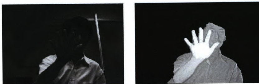
FIGURE 2.3: An example of an image containing depth information produced by the 3DV system's camera. Lighter areas are closer to the camera [22].
