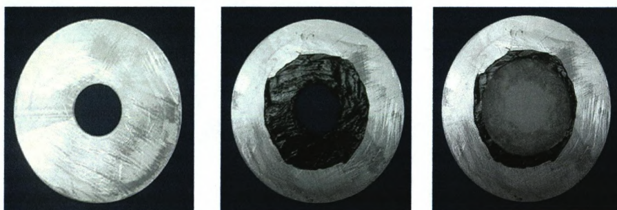
Fig. 1: Prepared membrane adhered on a support
