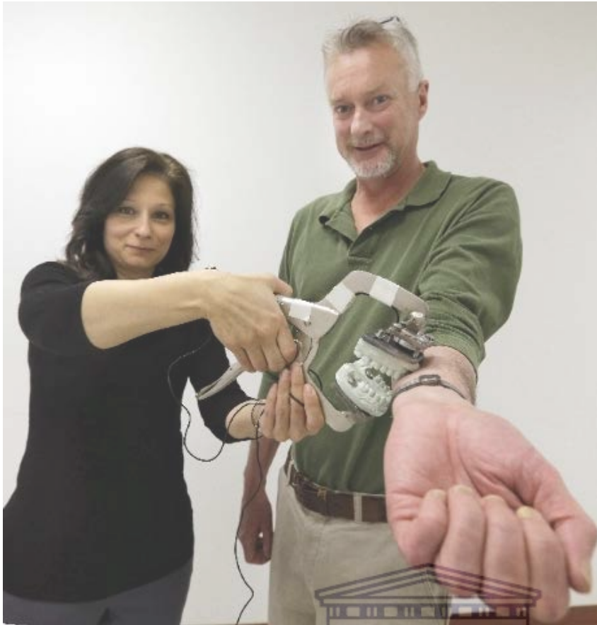
Figure 7: Mary and Peter Bush, research scientists at the University of Buffalo, NY, demonstrating a modified Vise-Grip Tool with attached dental mould that is used for test bites in humans or cadavers.
