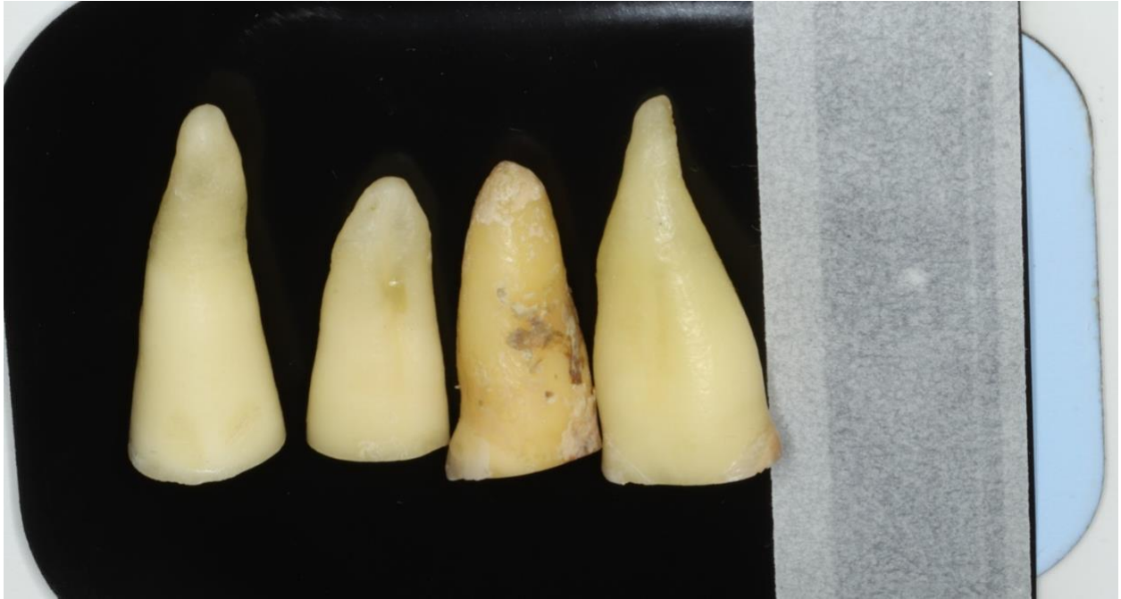
Figure 3. 5: Samples of specimens lined up on phosphor plates for imaging. A protective dark paper was used to over the phosphor plates to prevent scratching them.
