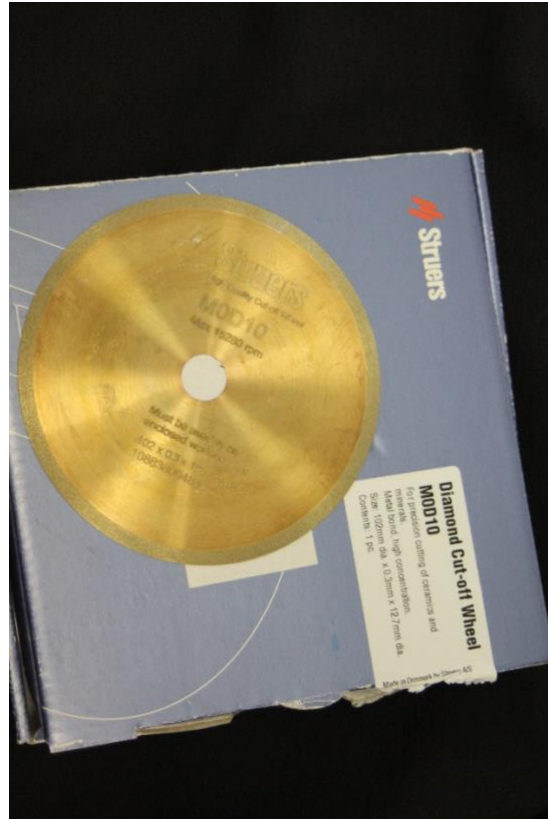
Figure 3.2: Left: Minitome machine Right: The struers diamond wheel used on the minitome machine to section the teeth at the CEJ
