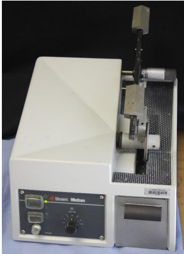
Figure 3.2: Left: Minitome machine Right: The struers diamond wheel used on the minitome machine to section the teeth at the CEJ
