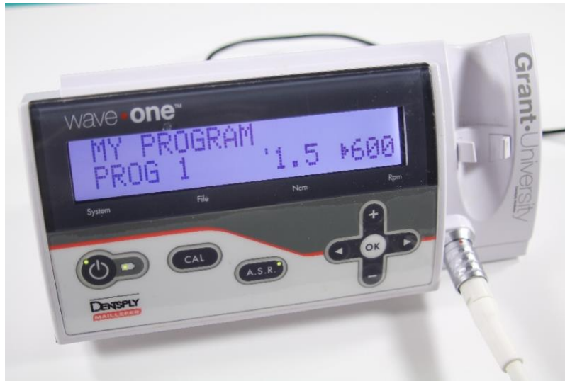
Figure 3.10: Endodontic motor with the torque and speed settings as required by the manufacturer of iRace treatment files used in the study
