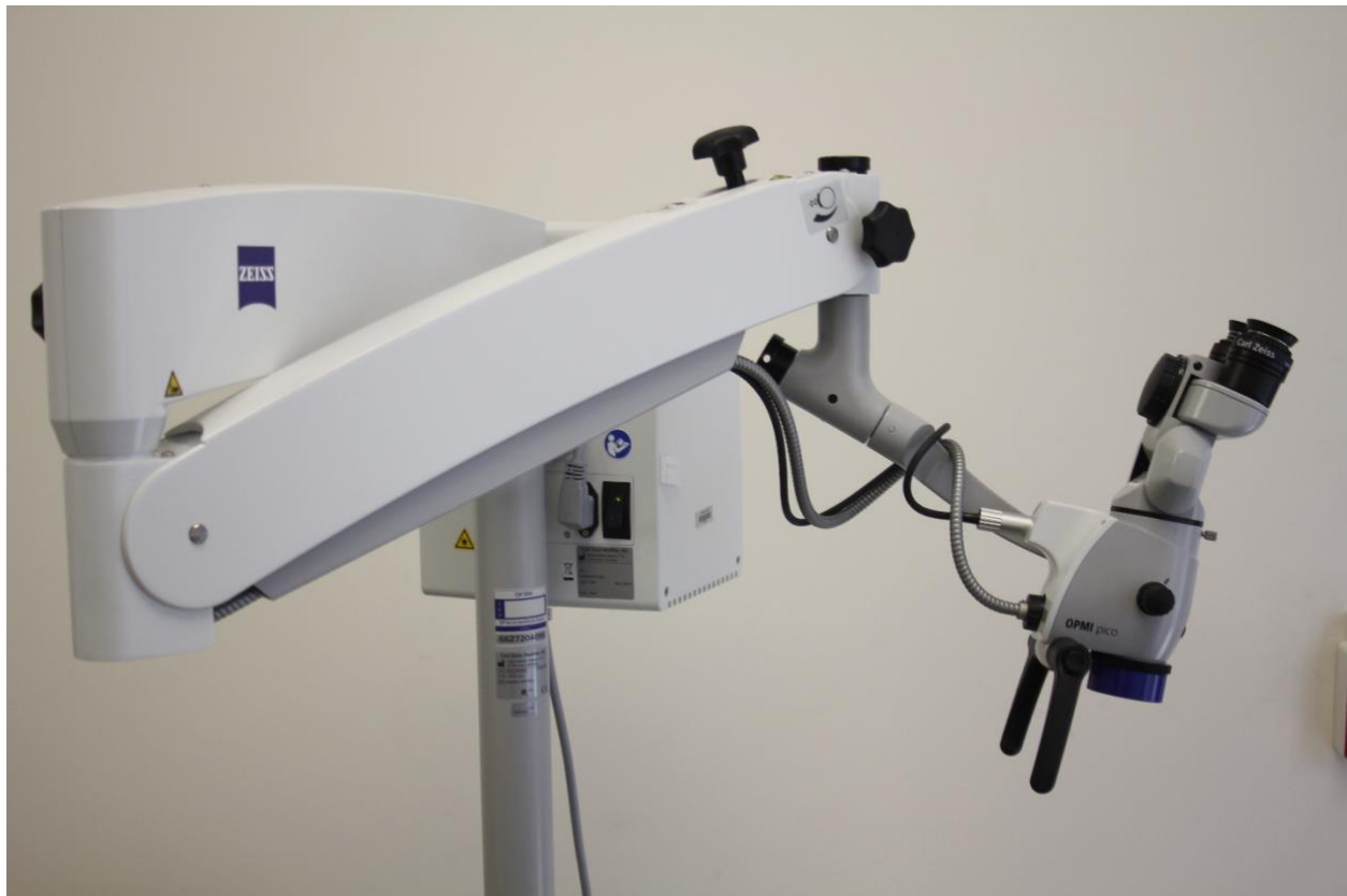
Figure 3.18: Dental Operating Microscope ((Zeiss S100 / OPMI pico, Carl Zeiss Meditec AG, Oberkochen, Germany).
