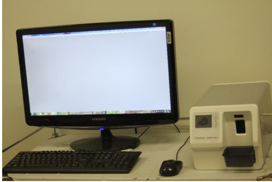
Figure 3.7: Digora scanner system (Orange, CA) used to process the exposed plates and project the images on the screen for viewing, manipulation of quality, storage and sharing.
