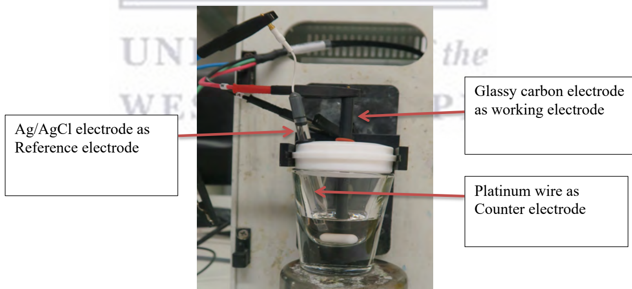
Figure 11: Example of a three-electrode system.
