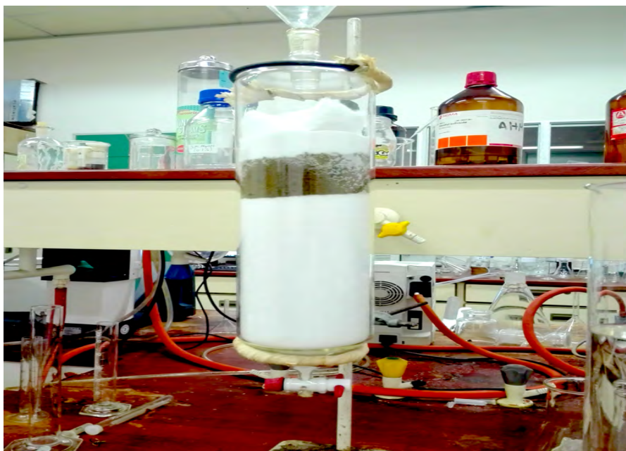
Figure 14: Open Column Chromatography set-up.
