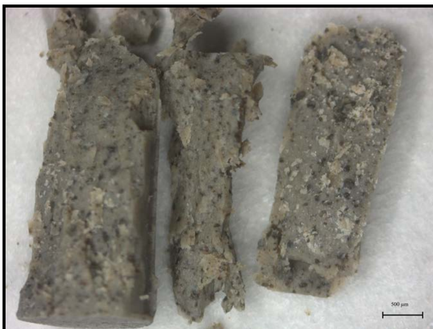
Figure 6.30: RSC10%ND-modified GIC sample from the compressive strength test with agglomerated nanodiamond particles visible
