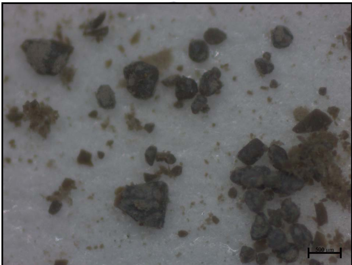
Figure 11.14: Agglomerated nanodiamond particles
