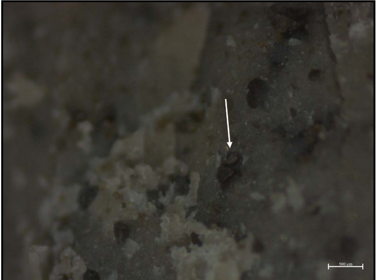
Figure 6.28: Fractured agglomerated particles within the RSC10%ND modified GIC during the compressive strength test (white arrow indicating nanodiamond agglomerated particle)
