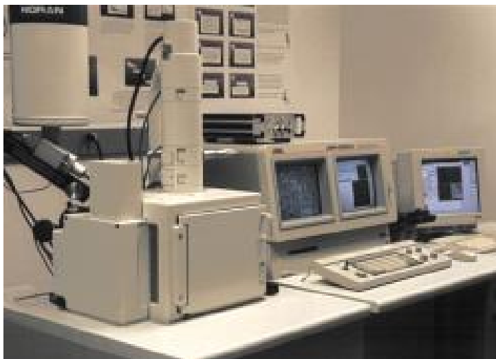
Figure 1.12: A typical SEM instrument, showing the electron column, sample chamber, EDS detector, electronics console, and visual display monitors.
