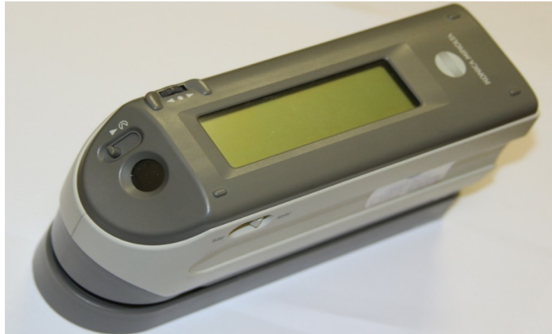
Figure 3.5: The CM-2600d spectrophotometer (Konica Minolta, Japan)
