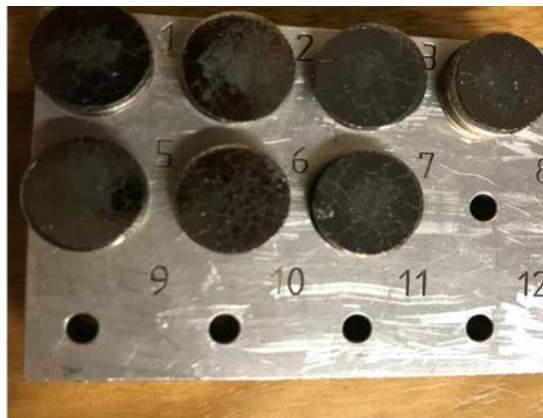
Figure 3.19: Samples sputter coated in gold.
