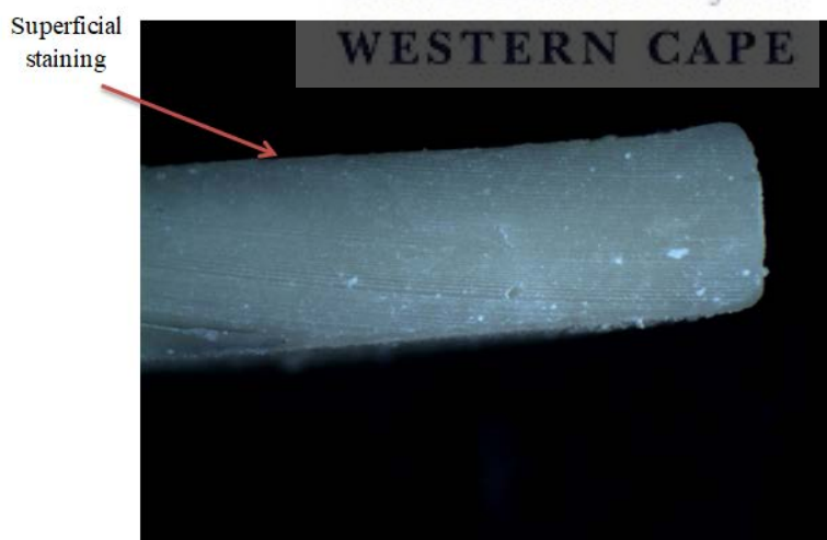
Figure 5.30: The polished surface of ChemFil™ Rock (top) showing superficial stain on its surface with mild penetrative staining.
