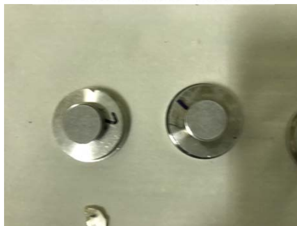
Figure 3.12: Aluminium stubs are prepared and numbered according to the material used.
