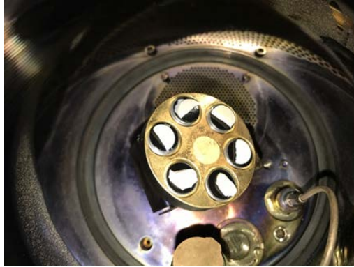
Figure 3.18: Samples in the Quorum Q150T ES High Resolution Sputter Coater (United Kingdom).
