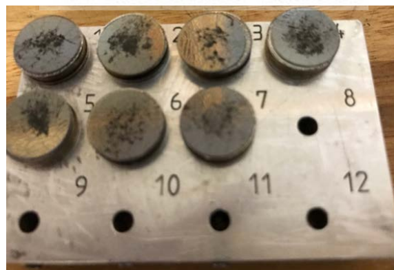
Figure 3.15: Sputter coated samples.
