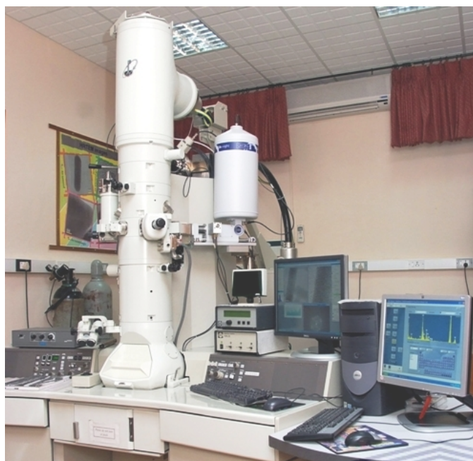
Figure 4: General layout of a HRTEM with EDAX (Dstuns.iitm.ac.in, 2019).
