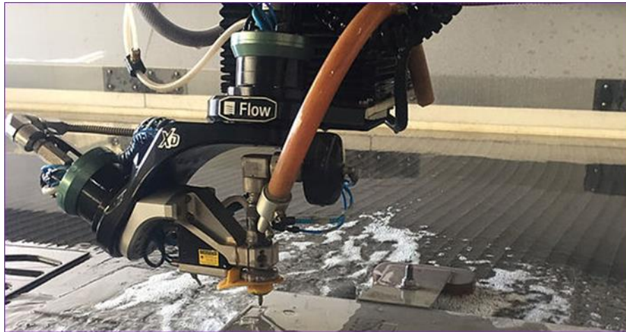
Figure 3.10: Water jet cutting machine for cutting of the holes (Flow Waterjets, USA)
