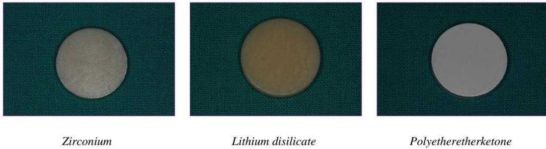
Figure 3.6: Sample discs - zirconium, lithium disilicate and polyetheretherketone
