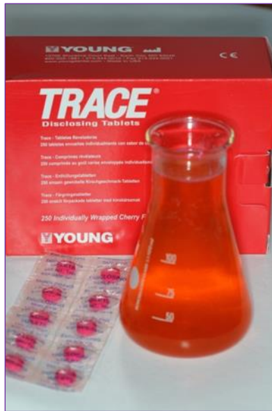
Figure 3.19: Disclosing solution (Trace Young, USA) used for staining of the biofilm
