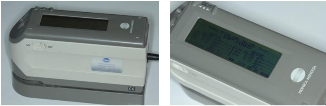
Figure 3.18: Spectrophotometer (Konica Minolta, Japan) used to measure the colour intensity of the samples
