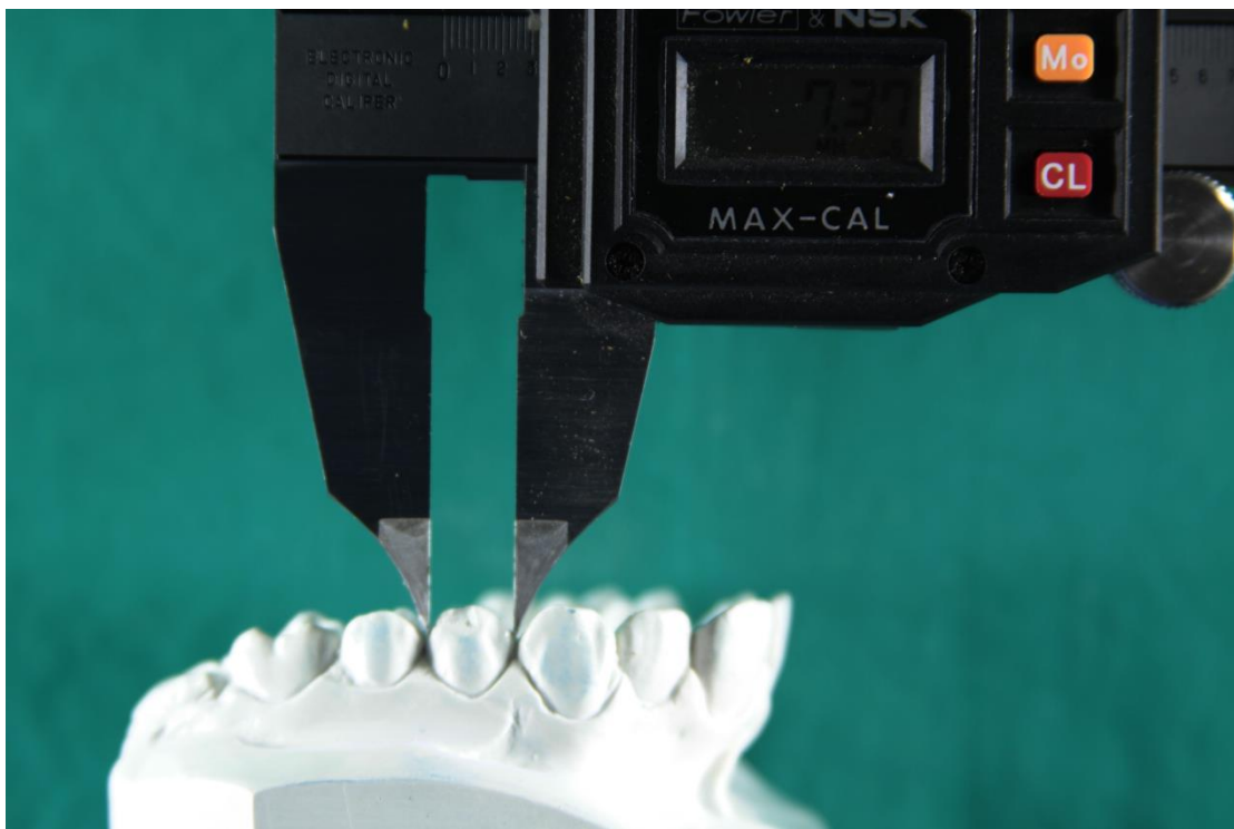
Figure 3.9 Measurement of plaster model with digital caliper
