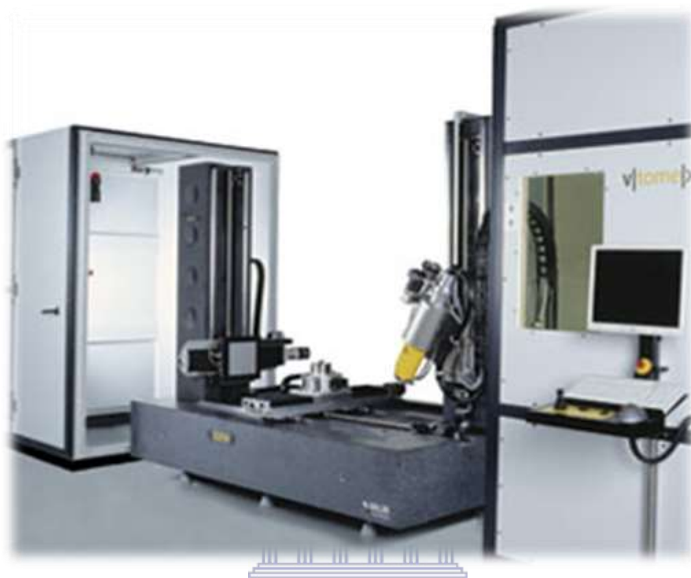
Figure 43: Micro-CT machine that was used to scan the root model A v|tome|x 240D (General Electric, MA, USA)
