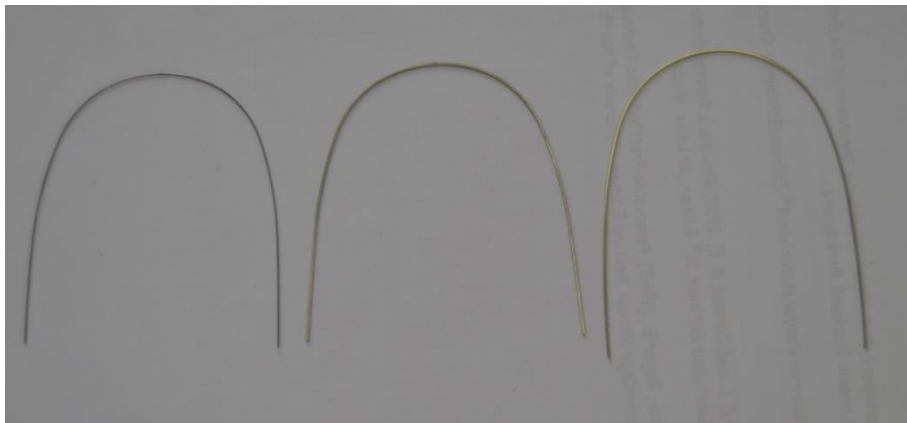
FIGURE 4: Three sections of archwires used: 0.016'' Ni-Ti, 0.019 x 0.025'' Ni-Ti and 0.019 x 0.025'' SS.
