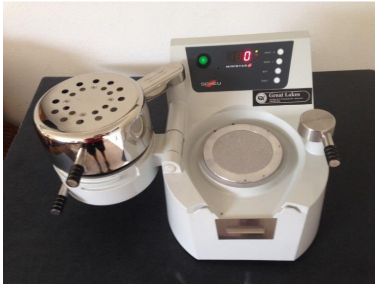
FIGURE 6: The Mini-Star S vacuum forming machine used to fabricate the template.
