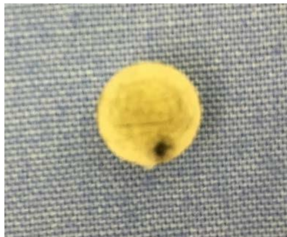
Figure 11: Specimen after removal from the mould showing marked top surface
