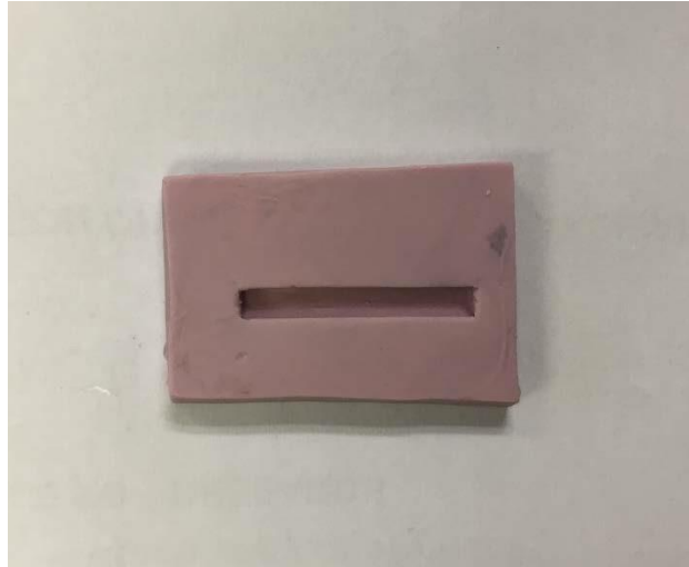
Figure 13: Mould used for flexural strength evaluation
