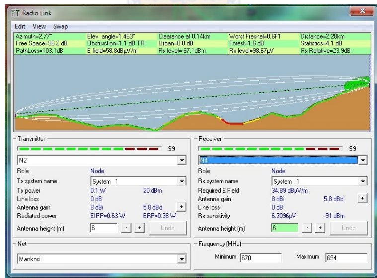
FIGURE 3.14: The radio characteristics in White Space as presented by Radio Mobile
