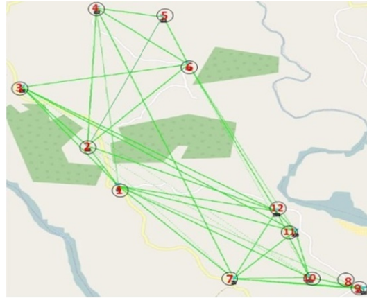
FIGURE 3.4: Zenzelini network: Connection between nodes in the White space frequency band
