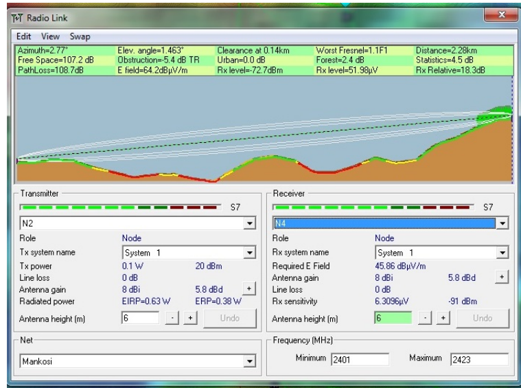
FIGURE 3.13: The radio characteristics in 2.4Ghz as presented by Radio Mobile
