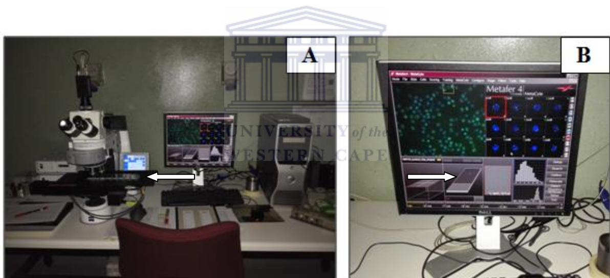
Figure 2.3: The Metafer 4 System set-up. (A) The complete Metafer 4 System (Metasystems) equipped with a 40x objective. The white arrow shows the stage of the inverted fluorescence microscope (Zeiss) that can contain 8 slides. (B) Detailed image to show precisely the location of the cell containing DNA DSBs, on the slide – indicated by the white arrow (iThemba LABS, Somerset West, South Africa).
