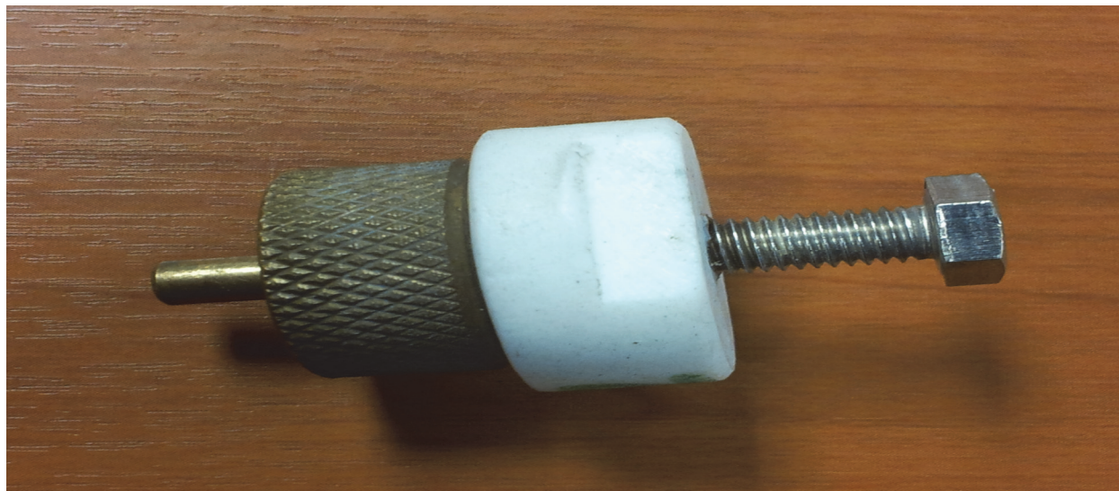
Figure 3.5.: Photograph of the coin cell used for electrochemical cycling testing.
