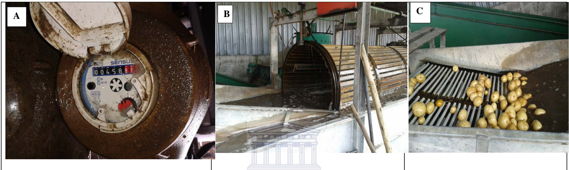
Figure 6.3: (A) Flow meter at installed at Modderfontein Farm used to measure water used to wash potatoes (B) Potato washing machine (C) Potatoes washing after harvest
