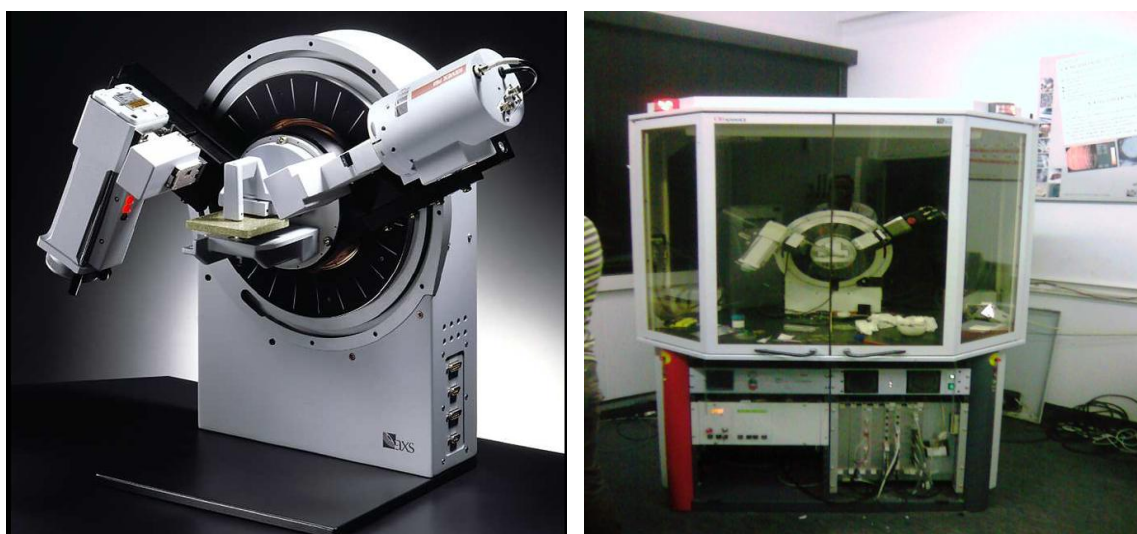
Figure 4.3: BRUKER D8 ADVANCE XRD instrument with pw3830 X-ray generator operated at 40Kv and 40mA.
