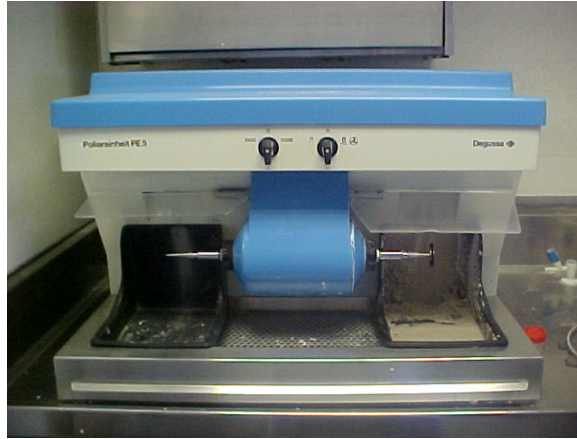
Figure 4.17 Dental lathe for polishing with a bristle brush
