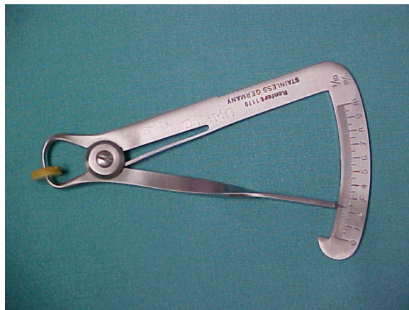
Figure 4.19 Renfert gauge measuring thickness of the specimen
