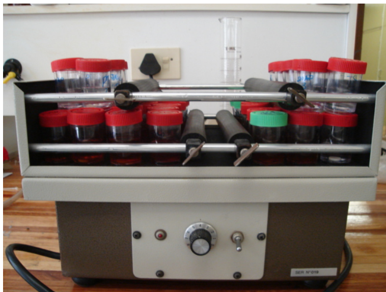
Figure 4.16: Specimen bottles in the orbital shaker moving at 30 revolutions per minute
