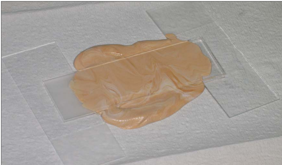
Fig 3.3: Using Silicone Putty to make a customized Silicone Mould
