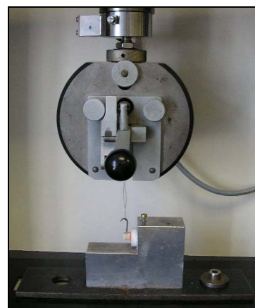
Fig.23: Upper member-hook holding nail
