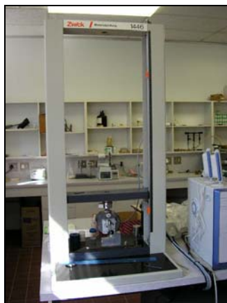
Fig.22: Zwick fatigue testing machine
