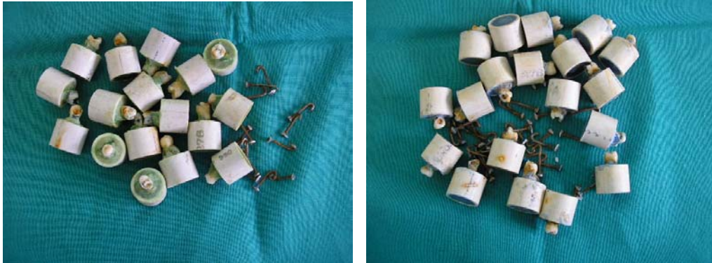
Fig.24: Debonding of nails after fatigue test: Group 1 and Group 2
