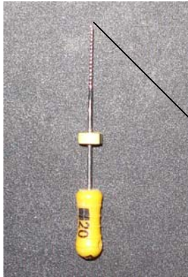
Fig 5.3 Fractured tip of K-File
