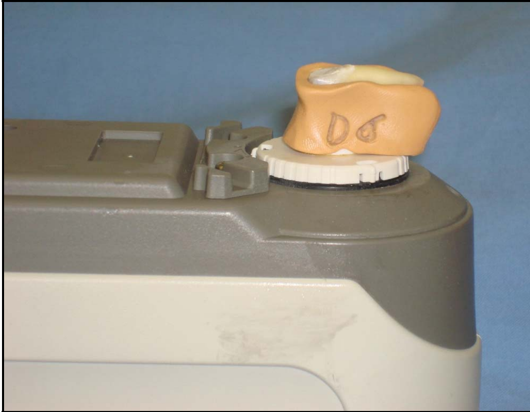
Figure 4.14 Spectrophotometer measuring tooth colour with index.
