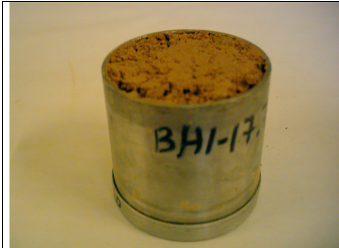
Berg river site 1: Depth= 17.7m:Malmesbury shales
