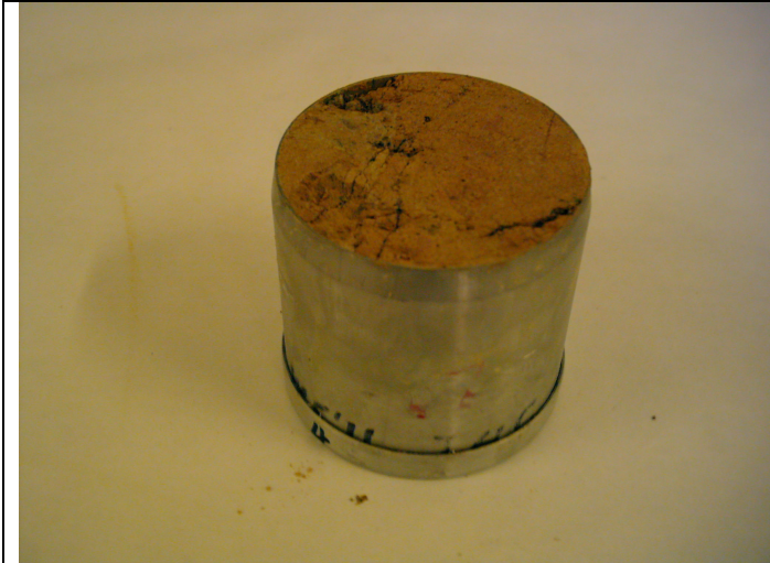
Berg river site 1: Depth= 11.5m:Malmesbury shales
