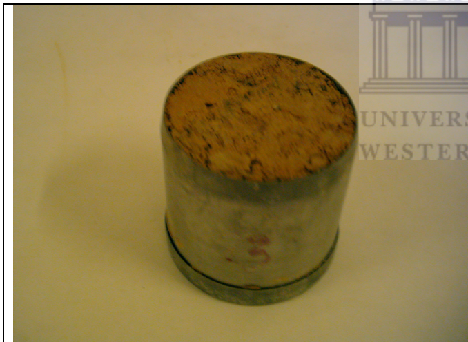
Berg river site 1: Depth=18.5m :Malmesbury shales
