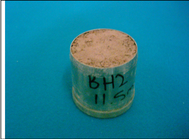
Berg river site 2: Depth= 11.5m: Malmesbury shales
