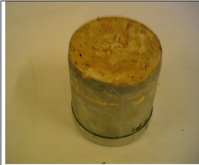
Berg river site 1: Depth= 1.8m: Clay
