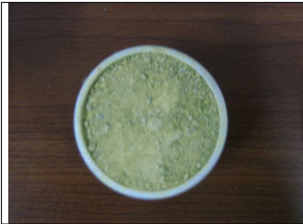
Berg river site 3: Depth= 7.5m Malmesbury shale
