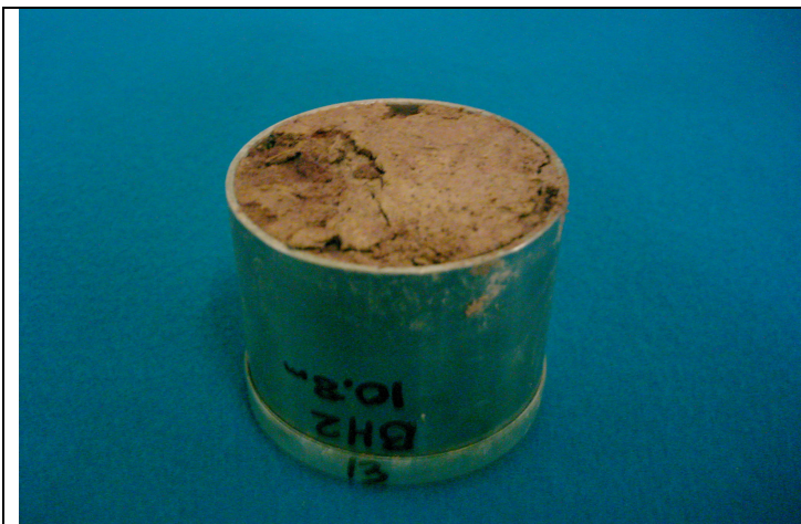
Berg river site 2: Depth= 10.8m: Malmesbury shales
