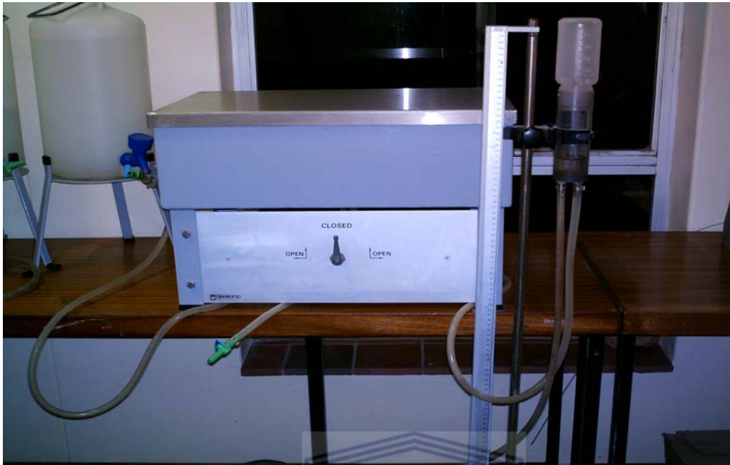
Figure 3.3: Eijkelkamp Sandbox setup in the Hydraulics lab (UWC)
