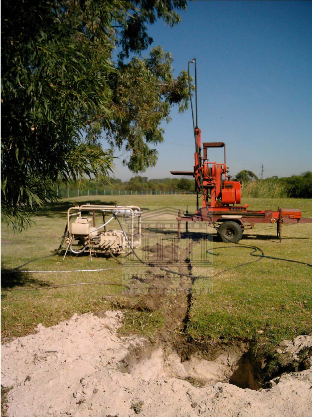
Figure 3.2: Illustrating the drilling setup (iThemba site 1) which includes: the drilling machine, generator, and 1m 2 hole (where mixing 0.5%EZEEMIX with water occurred).
