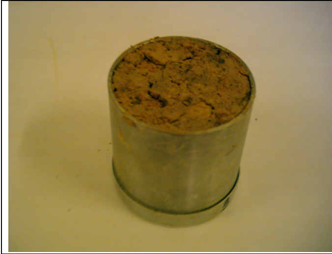
Berg river site 1: Depth= 8.5m :Malmesbury shales
