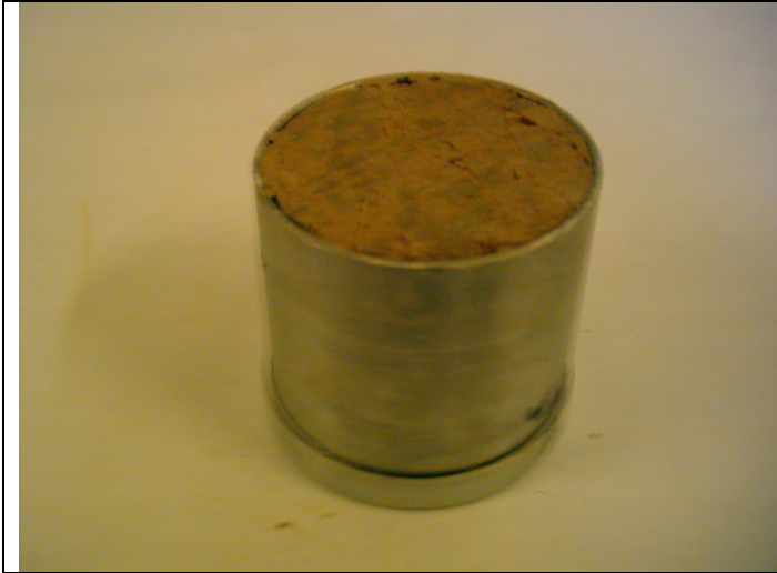
Berg river site 1: Depth=15.3m:Malmesbury shales
