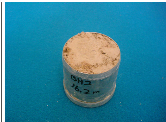
Berg river site 2: Depth= 16.2m Malmesbury shales
