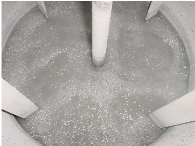
Figure 2.2. A top view of the pilot rig, showing the stirring of FA and AMD.
