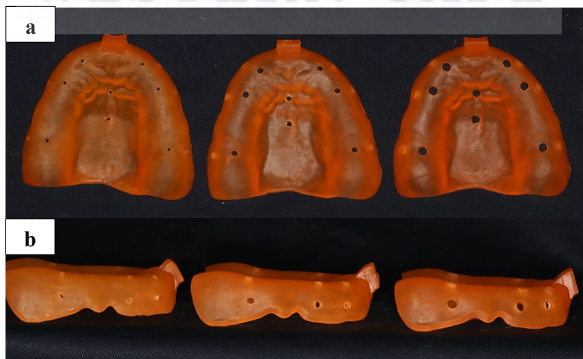
Figure 19: Tray design 2 (14 relief holes) with 1mm (left), 2mm (middle) and 3mm (right) relief hole diameters, a) alveolar ridge and palate relief holes, b) posterior and anterior buccal relief holes.
