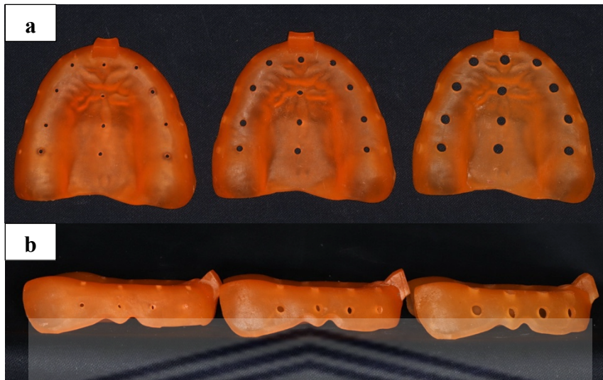
Figure 20: Tray design 3 (21 relief holes) with 1mm (left), 2mm (middle) and 3mm (right) relief hole diameters, a) alveolar ridge and palate relief holes, b) posterior and anterior buccal relief holes.
