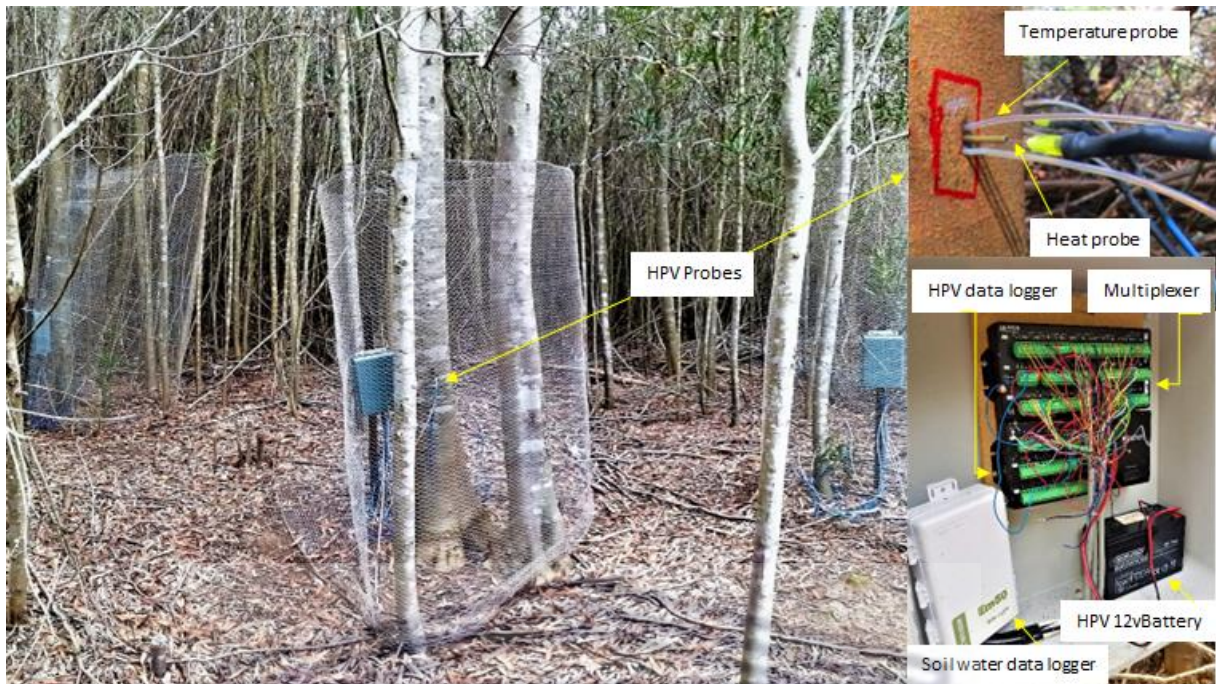
Figure 4.4: HPV system comprising heat and temperature probes connected to a safety box that enclosed a multiplexer, datalogger, and a 12V battery. The soil water data logger was also enclosed in the box to protect soil water sensors installed at various depths close to the selected trees.
