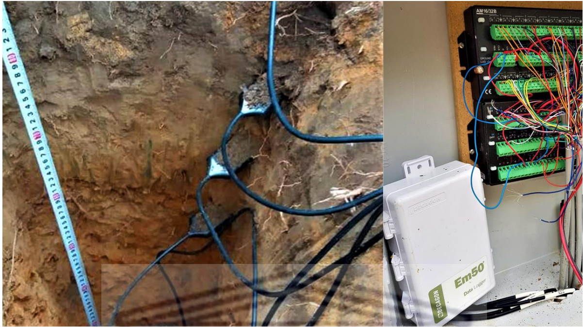
Figure 5.2: Decagon soil water sensors installed at various depths (left) and the Em50 data logger (right).
