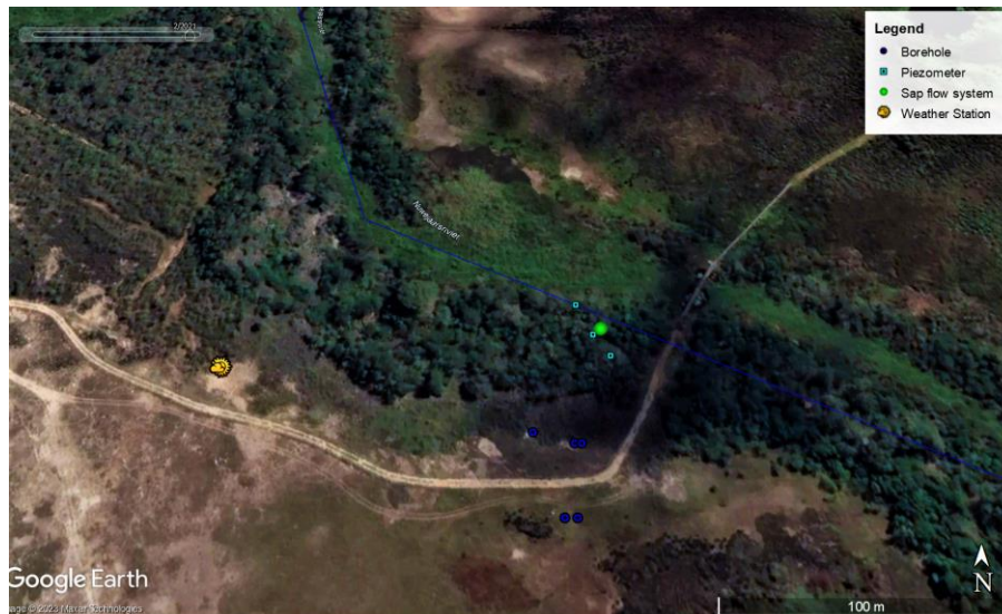
Figure 2.7: Moddervlei's monitoring set-up. Soil water sensors were in proximity to the sap flow (Source: Google Earth Image of 6th February 2021).
