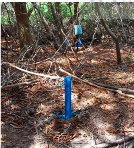
Figure 5.3: Typical hand-augured piezometer (left) and drilled boreholes (right) at sites to monitor water table fluctuations.
