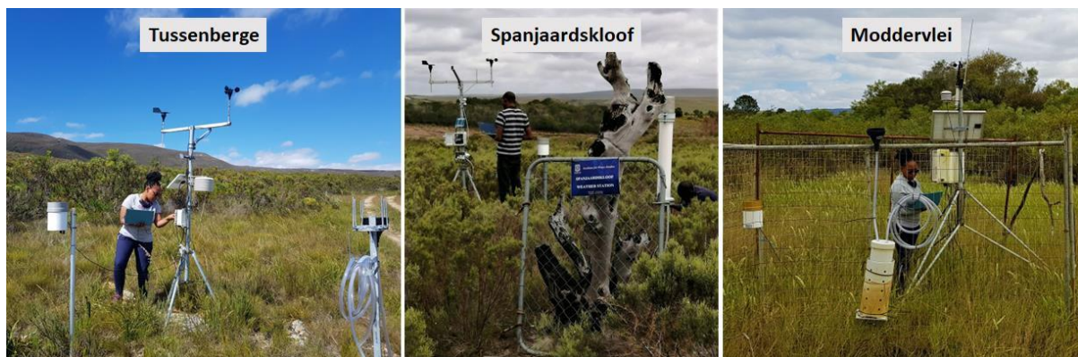
Figure 4.2: Automatic weather stations established at the sites.
