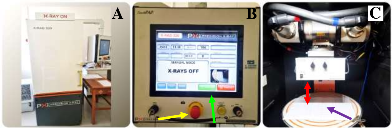
Figure 29: PXi Precision X-ray machine at NRF iThemba LABS. A) The overview of the X-ray machine. B) The control panel. The green arrow indicates the start button of the X-ray and the yellow button indicated the emergency stop button for the X-ray. C) T25 flask in the field view indicated by the purple arrow and the red arrow indicate the SSD.
